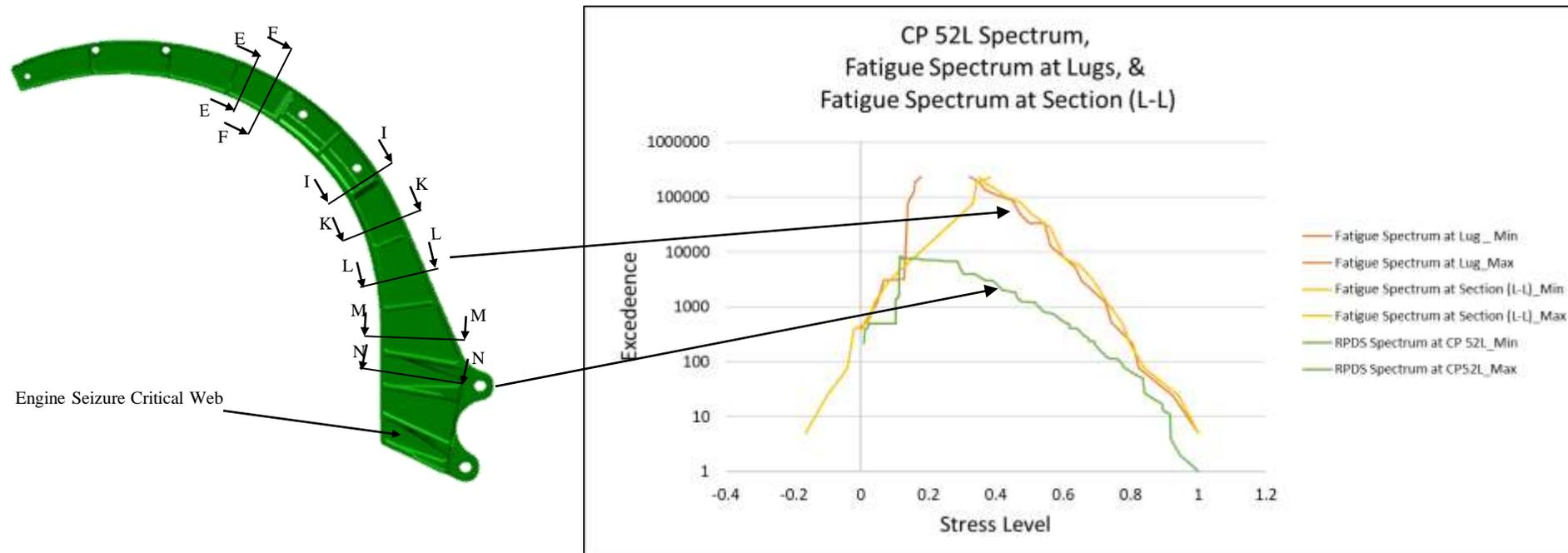
A comparison between the three spectrum show that the fatigue spectrum (6,000 hour spectra) has more max stress events then RPDS, which is what would be expected. It also shows that there is similar number of max peaks events for the fatigue spectrum of lug as compared to Section L-L.
