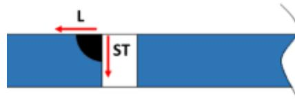
Forging Grain Direction in flanges
