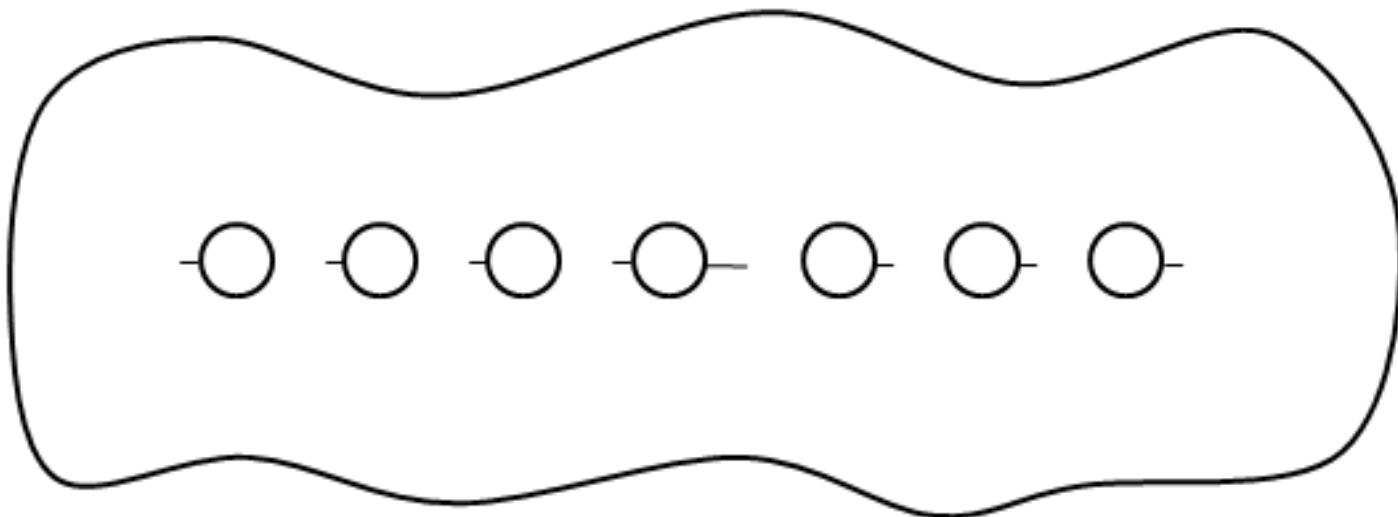
Single, primary crack with secondary cracks at each hole in a row of holes in an infinite plate
